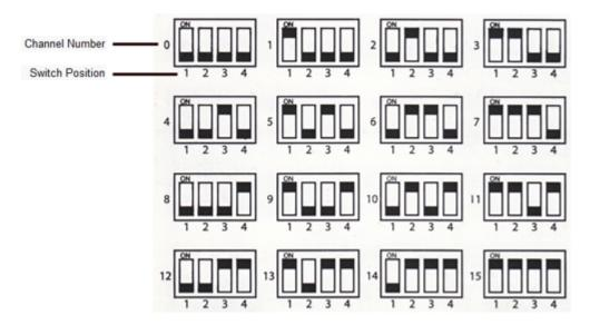
The Black Squares are the Position of the Dip Switch. Make all Dips match the Blacken Squares as in the Chart. Ex: The above Setting shows for Channel 0 - All Dip Switches must be in the Down Position - for 457.5875MHz.
