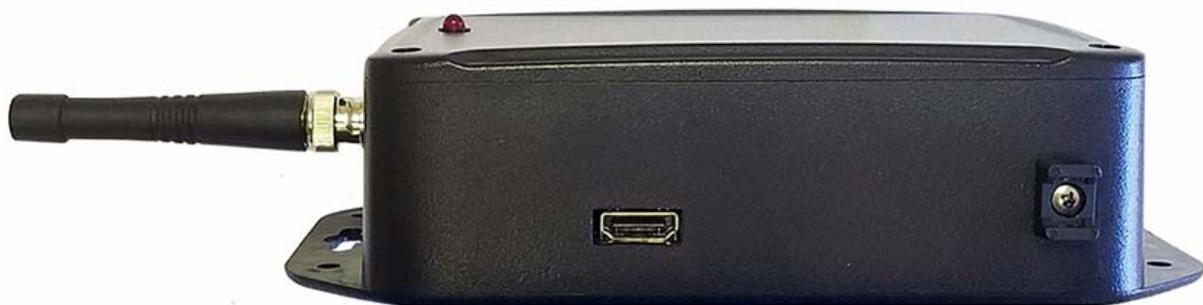
**Figure 5 - DAV Left Side View with HDMI Connector and Tie Down**
