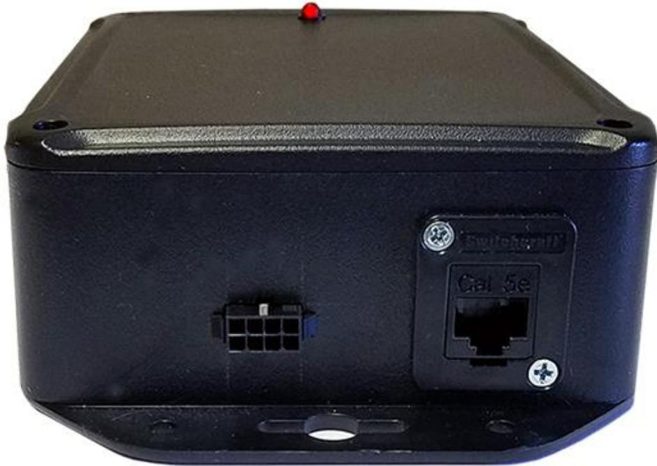
Figure 4 - DAV Bottom View with Power/Programming/Output Control Connector and Ethernet Jack
