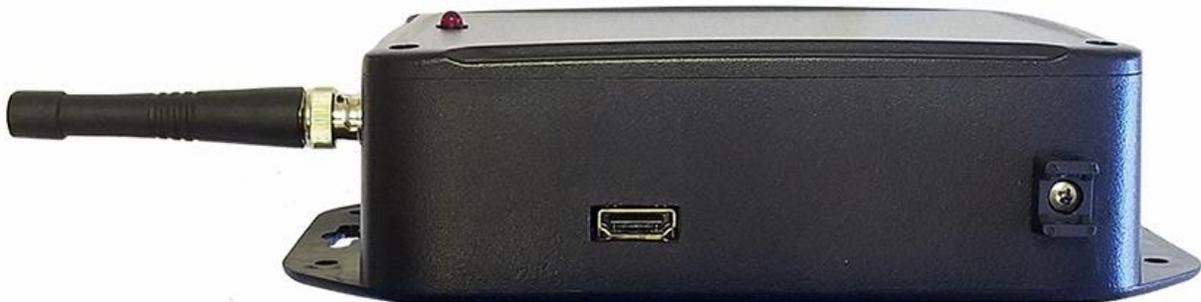
Figure 5 - DAV Left Side View with HDMI Connector and Tie Down
