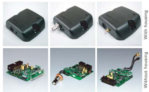
Onboard antenna      BNC connector      OSX connector
